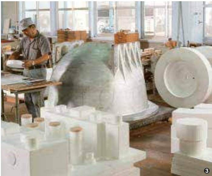
① Planning meeting ② CAD product design ③ Wooden mold model / Foamed mold model
